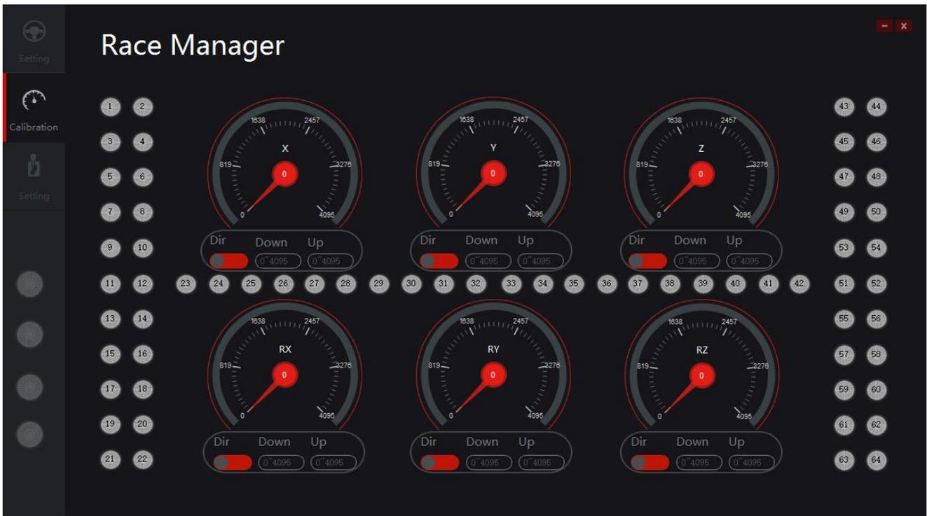
**Motor setting interface**, which can view the basic information and system status of race manager.
